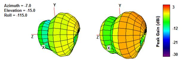
Figure 8. 3D Radiation Pattern at 1710 MHz (left), 1805 MHz (right) of the TG19 Antenna.
