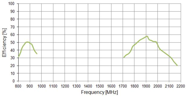
Figure 4. Efficiency of the TG19 antenna.
