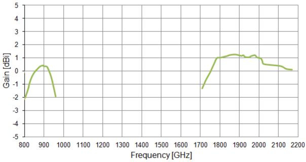
Figure 5. Peak Gain of the TG19 Antenna.
