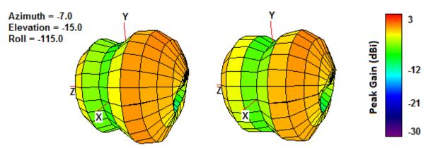
Figure 9. 3D Radiation Pattern at 1910 MHz (left), 1990 MHz (right) of the TG19 Antenna.
