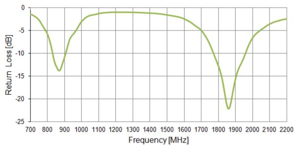
Figure 2. Return loss of the TG19 Antenna.
