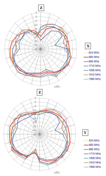
Figure 10. 2D Radiation Pattern of the TG19 Antenna.
