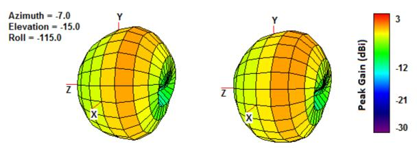
Figure 7. 3D Radiation Pattern at 850 MHz (left) 915 MHz (right) of the TG19 Antenna.
