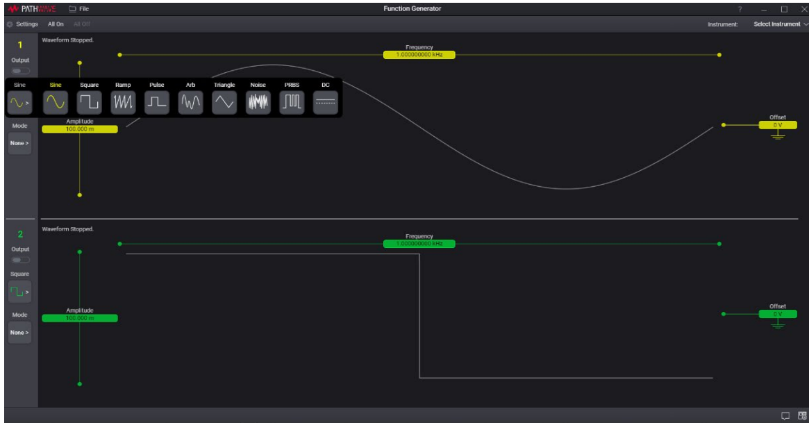
Figure 5. Select and configure your required waveform
