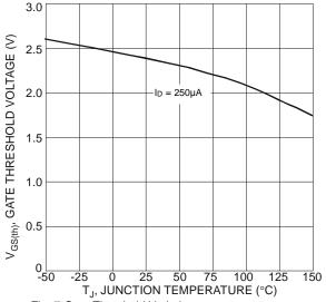
Fig. 7 Gate Threshold Variation vs. Junction Temperature
