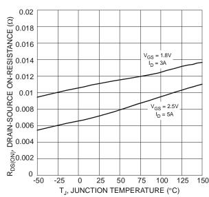
Figure 7 On-Resistance Variation with Temperature
