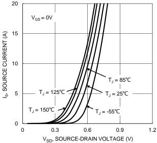
Figure 9. Diode Forward Voltage vs. Current
