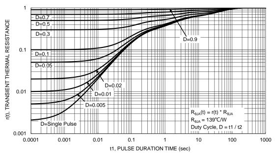
Figure 13. Transient Thermal Resistance
