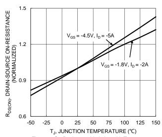
Figure 6. On-Resistance Variation with Temperature
