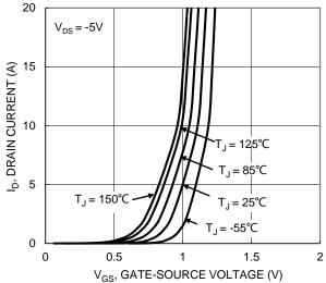
Figure 2. Typical Transfer Characteristic
