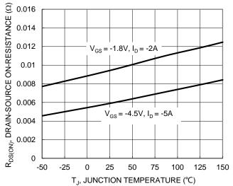
Figure 7. On-Resistance Variation with Temperature
