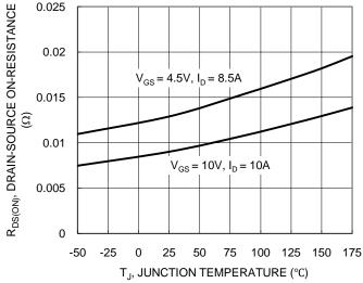
Figure 7. On-Resistance Variation with Temperature
