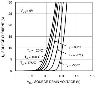
Figure 9. Diode Forward Voltage vs. Current
