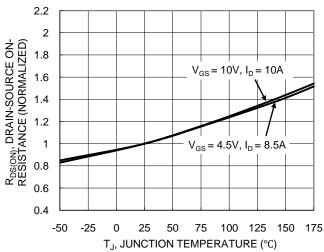
Figure 6. On-Resistance Variation with Temperature
