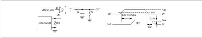
Figure 4. Driver Enable and Disable Times (t<sub>DZH</sub>, t<sub>DHZ</sub>)
