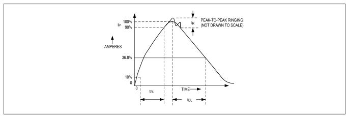
Figure 11. Human Body Current Waveform
