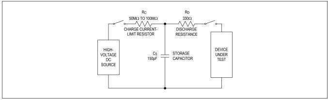
Figure 12. IEC 61000-4-2 ESD Test Model
