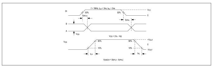
Figure 3. Driver Propagation Delays
