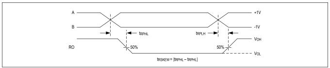
Figure 7. Receiver Propagation Delays
