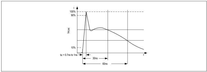
Figure 13. IEC 61000-4-2 ESD Generator Current Waveform
