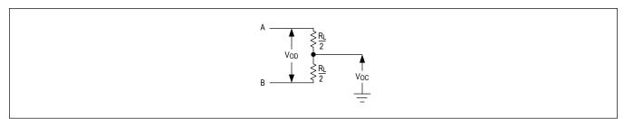
Figure 1. Driver DC Test Load
