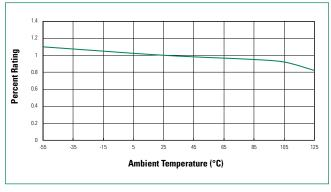
Note: Re-rating depicted in this curve is in addition to the standard derating of 25% for continuous operation.
