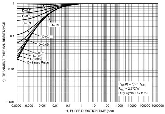
Figure 13. Transient Thermal Resistance
