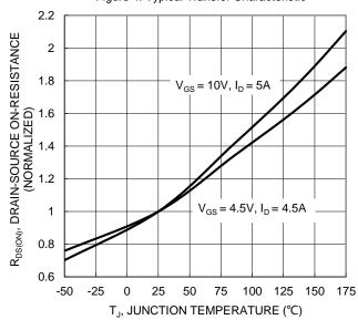
Figure 6. On-Resistance Variation with Junction Temperature
