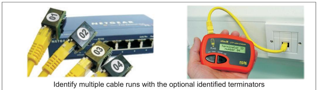
Identify multiple cable runs with the optional identified terminators
