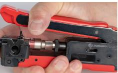
Using specially designed jaws to hold connectors in place while compressing, this **PATENTED** CTF-360 is designed to hold and compress connectors requiring a full 360 degree support. Perfect tool for short F connectors for RG59/6 cables and F connectors for RG7/11 cables. This tool also features the following:
