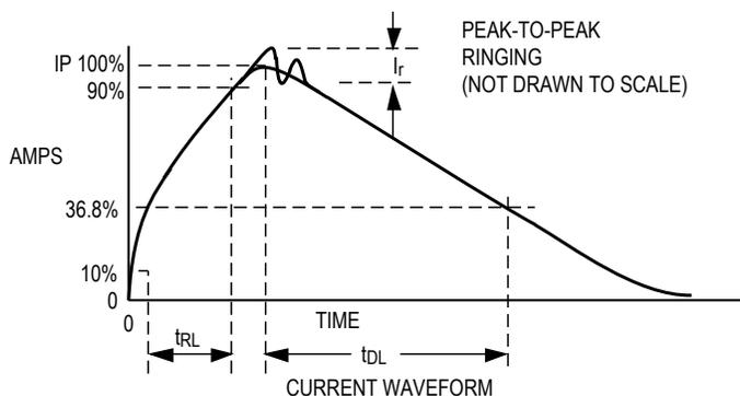
Figure 10. Human Body Current Waveform
