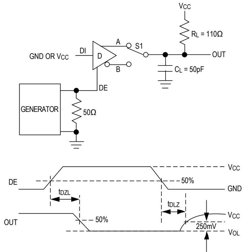
Figure 5. Driver Enable and Disable Times ( $t_{DZL}$ ,  $t_{DLZ}$ )
