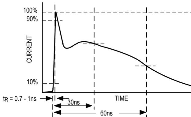
Figure 12. IEC 61000-4-2 ESD Generator Current Waveform
