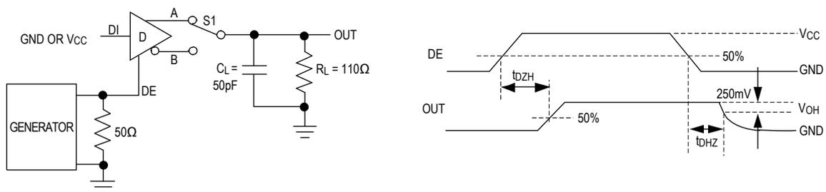
Figure 4. Driver Enable and Disable Times ( $t_{DZH}$ ,  $t_{DZL}$ )
