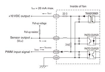
$$\begin{split} &V_{\text{CE}} = +27.6 \text{ V max.} \\ &I_{\text{C}} = 10 \text{ mA max.} \left[ V_{\text{OL}} \!\!=\!\! V_{\text{CE}} \left( \! \text{SAT} \right) \!\!=\!\! 1 \text{ V max.} \right] \\ &Pull-up \ resistor = 5 \ k\Omega \ max. \end{split}$$
