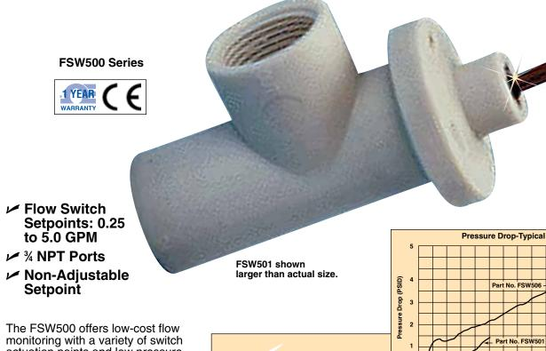
actuation points and low pressure drop. With their polypropylene or stainless steel wetted parts, these switches are suitable for a wide range of chemical and temperature requirements. The FSW500 is ideal for cooling of equipment such as welders and lasers. A J-box version with a 5 A relay is also available.
