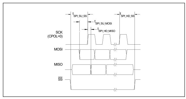
Figure 5: Timing characteristics
