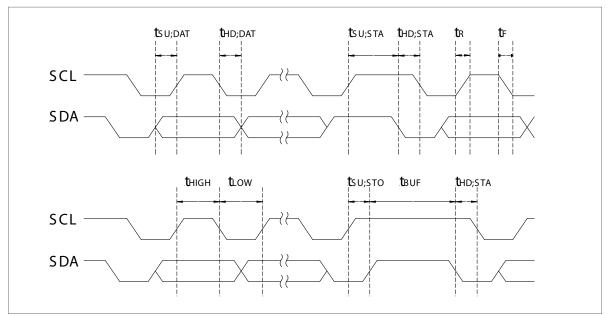
Figure 2. Timing Characteristics
