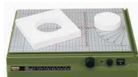
Crosscuts are achieved by means of a simple yet efficient solution: secure drawing-pin to table by means of tape, it serves as a fixed centre.
