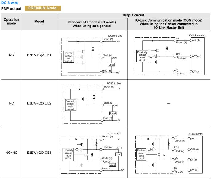
In the IO-Link mode, the cord between the IO-Link master and sensor must have a length of 20 m or less.
