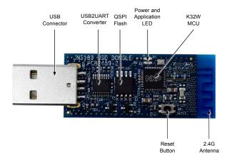
Figure 1: OM15080-K32W Board Components
