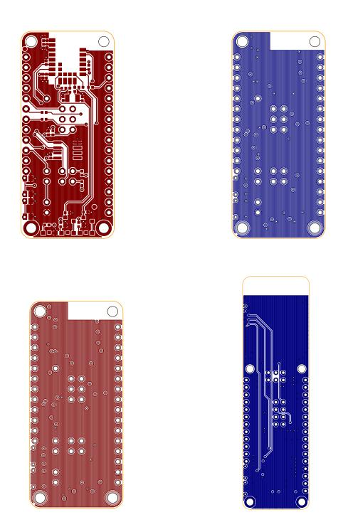
Figure 7: Top, bottom and internal layers
