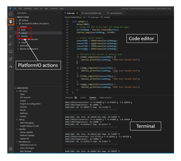
Figure 9: Running the quick start example
