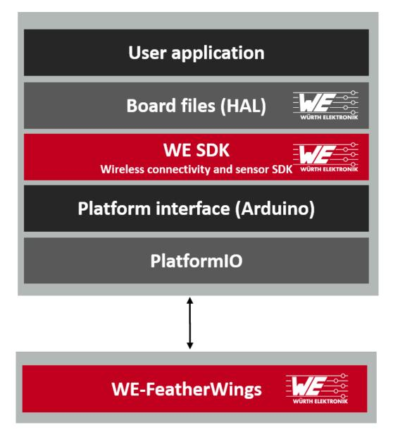
Figure 8: Software architecture
