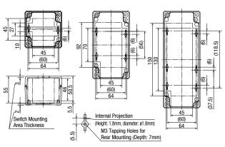
Choose an enclosure in consideration of switch's depth behind the panel and the mounting centers of the adjacent switches.
