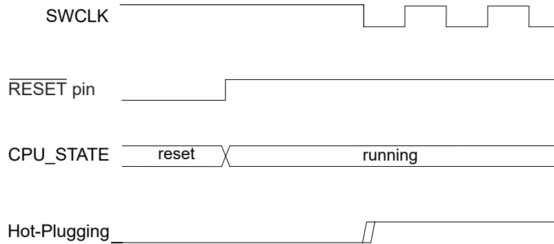
Figure 13-3. Hot-Plugging Detection Timing Diagram
