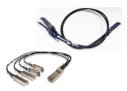
Volex's QSFP+ to 4x SFP+ passive copper breakout Direct Attach Cable is a cost-effective alternative to optical modules for short reach high speed interconnects. The cable assembly enables breakout of 40GbE QSFP+ port to 4x 10GbE SFP+ ports, optimizing data center solutions for interconnecting 40G Ethernet switch port to 4x 10G server ports.
