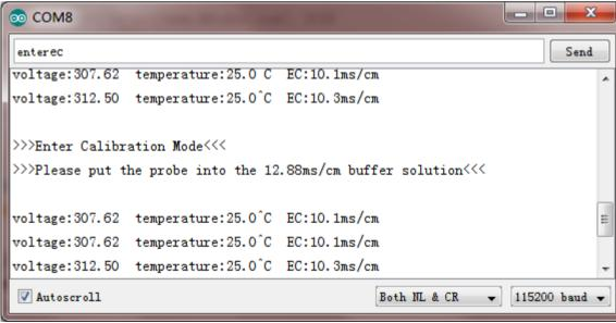
ii. Input CALEC commands to start the calibration. The program will automatically identify the standard buffer solution of 12.88ms/cm.
