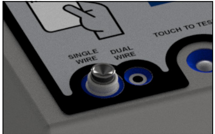
Figure 8. Completed installation of the plunger and spring assembly
