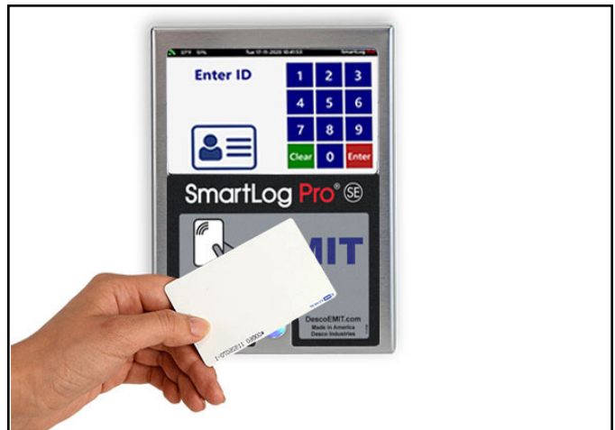
Figure 15. Holding a proximity badge in front of the RFID icon on the SmartLog Pro® SE
