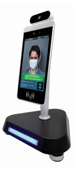
Base thickness: 1.5 inches (3.8 cm) (2) USB ports Base with adjusting screws Blue light strip Cold-rolled plate painting
