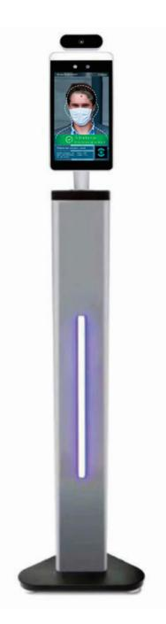
Height: 43.3 inches (110 cm) (2) USB ports Base with adjusting screws Blue light strip Cold-rolled plate painting
