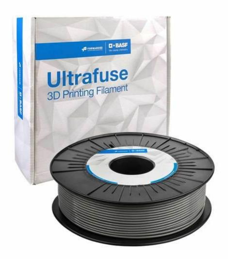
Ultrafuse 316L combines greater freedom of design with a low total cost of ownership. 3D-printed parts acquire their final properties, for example in terms of hardness and strength, through a debinding and sintering process developed by BASF, which has emerged as the industry standard. As a filament, Ultrafuse 316 L is 80% stainless steel and has a 20% polymer content which allows for easy printing on many open FFF desktop printers.
