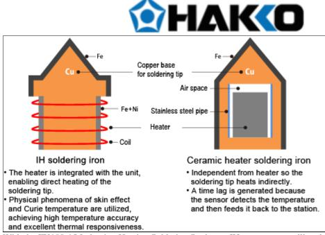
With the FX100-15 Induction Heating Soldering Station or IH system, controlling the temperature of the soldering iron is easy
