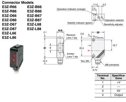
Note: The lens for the E3Z-D 1/D 6/L /B is red. The lens for the E3Z-D 2/D 7 is black.
