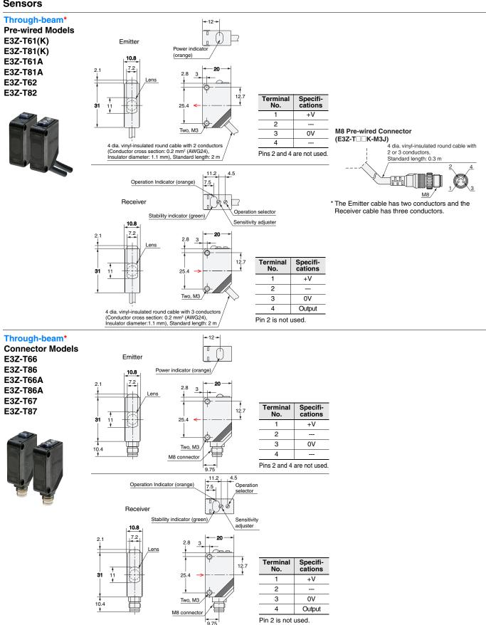
\* Models numbers for Through-beam Sensors (E3Z-TIDD) are for sets that include both the Emitter and Receiver. The model number of the Emitter is expressed by adding "-L" to the set model number (example: E3Z-T61-L 2M), the model number of the Receiver, by adding "-D" (example: E3Z-T61-D 2M.) Refer to Ordering Information to confirm model numbers for Emitter and Receivers.
