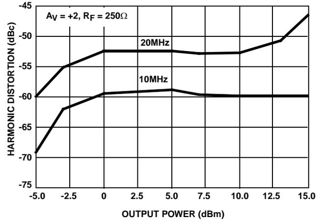
FIGURE 31. 3rd HARMONIC DISTORTION vs P<sub>OUT</sub>
