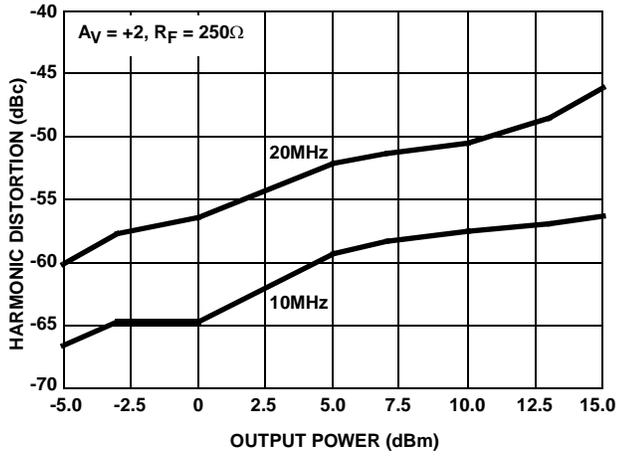
FIGURE 30. 2nd HARMONIC DISTORTION vs P<sub>OUT</sub>
