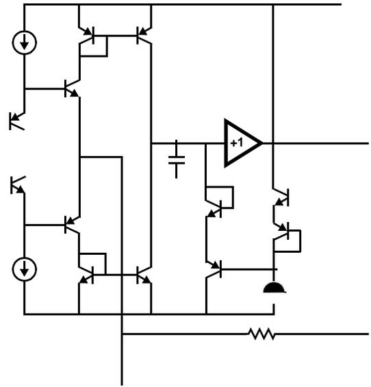
This current is mirrored onto the high impedance node ( $Z$ ) by  $Q_{X3} - Q_{X4}$ , where it is converted to a voltage and fed to the output via another unity gain buffer. If no limiting is utilized, the high impedance node may swing within the limits defined by  $Q_{P4}$  and  $Q_{N4}$ . Note that when the output reaches its quiescent value, the current flowing through  $-IN$  is reduced to only that small current ( $-I_{BIAS}$ ) required to keep the output at the final voltage.
