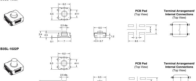
**Note:** Unless otherwise specified, a tolerance of  $\pm 0.2$  mm applies to all dimensions.
