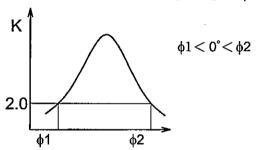
Contrast ratio K vs viewing angle  $\phi$
