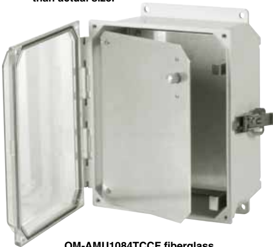
OM-AMU1084TCCF fiberglass enclosure with molded-in hinge, clear polycarbonate window and padlocking twist latch. Shown with OM-HFPU108, front dead panel sold separately.
