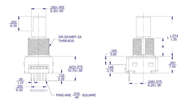
GENERAL TOLERANCE:  $\frac{\pm.010 \text{ inch}}{\pm 0.25 \text{ mm}}$
