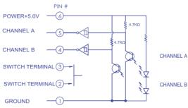
\*Schmitt trigger and pull-up resitor (4.7K $\Omega$ ) are integrated inside CTS optical encoder, so it's not necessary to have external pull-up resistors for application circuit.
