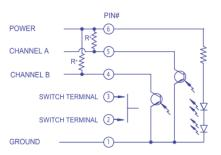
\*Product will function properly with external 2.2K $\Omega$  pull up resistors.
