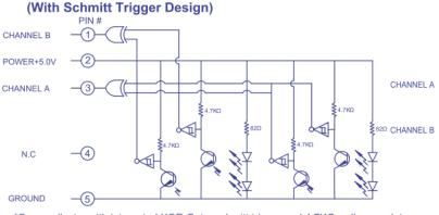
\*Open collector with integrated XOR Gate, schmitt trigger and  $4.7K\Omega$  pull-up resistor are inside CTS optical encoder, so it's not necessary to have external pull-up resistors for application circuit.
