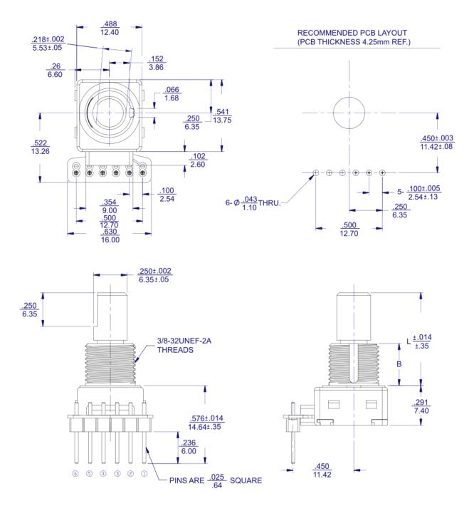
GENERAL TOLERANCE:  $\frac{\pm .010 \text{ inch}}{\pm 0.25 \text{ mm}}$
