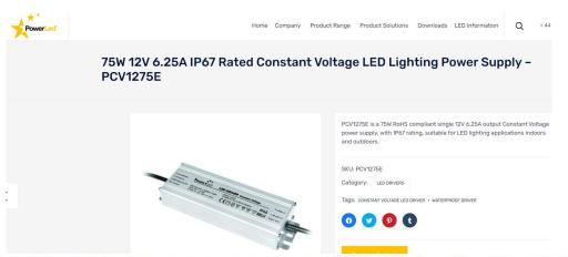
PCV1275E is a 75W RoHS compliant single 12V 6.25A output Constant Voltage LED Lighting Power Supply with IP67 rating, suitable for LED lighting applications indoors and outdoors. PCV1275E has 100-240V input voltage, is of Class II design and offers cooling via free air convection.
