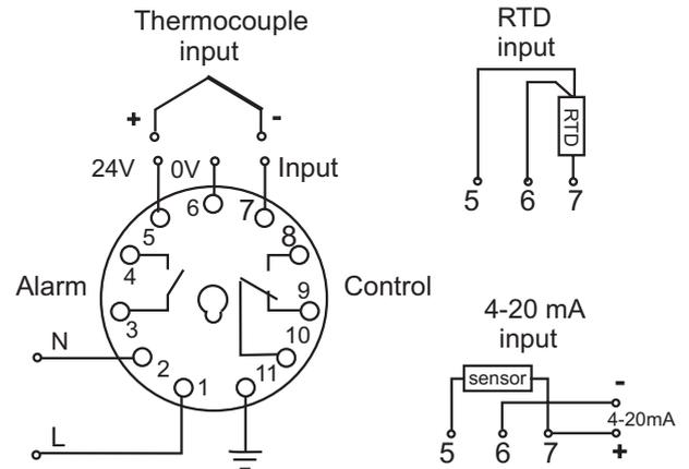
**Note :** When pin 11 and the sensor are both earthed, the DTC410 will display OPN and will not operate correctly. For 24V models use an isolated or non-earthed sensor.
