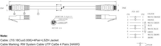
Cable Marking: RW System Cable UTP Cat5e 4 Pairs 24AWG
