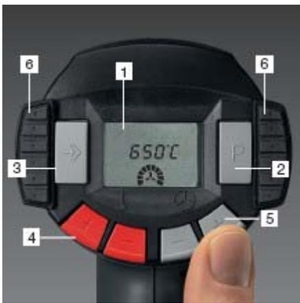
1. Visual display of temperature and speed on LCD
