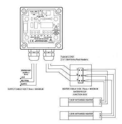
Technical Specification Mains Voltage Operation Current Power Consumption Set Time Period 1 to 3 Temperature trip point Max load at 20°C ambient Max Unit Operating Temperature IP Rating Gland Diameter (Fitted) 2 Lamp Installation WARNING: THIS UNIT MUST BE EARTHED
