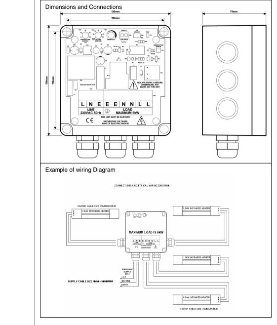
Check all wiring - particularly the line and load connections and make cure the cable alande
