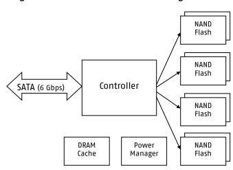
Figure 1: F-66 CFast Functional Block Diagram
