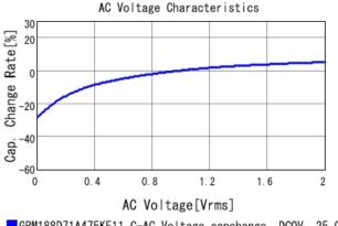
GRM188D71A475KE11 C-AC Voltage capchange, DCOV, 25.0d
