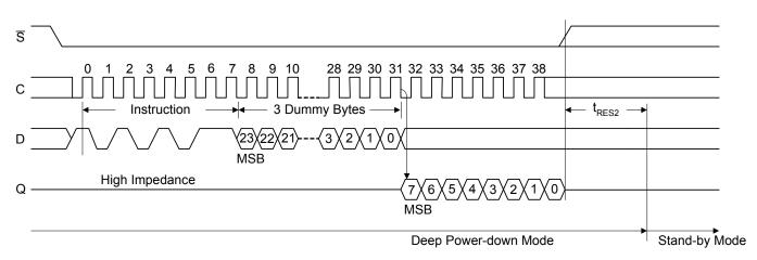
Note: The value of the 8-bit Electronic Signature, for the A25L80P, is 13h.
