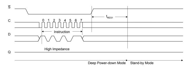
Driving Chip Select (<sup>S</sup>) High after the 8-bit instruction byte has been received by the device, but before the whole of the 8-bit Electronic Signature has been transmitted for the first time (as shown in Figure 16.), still insures that the device is put into Stand-by Power mode. If the device was not previously in the Deep Power-down mode, the transition to the Stand-by Power mode is immediate. If the device was
