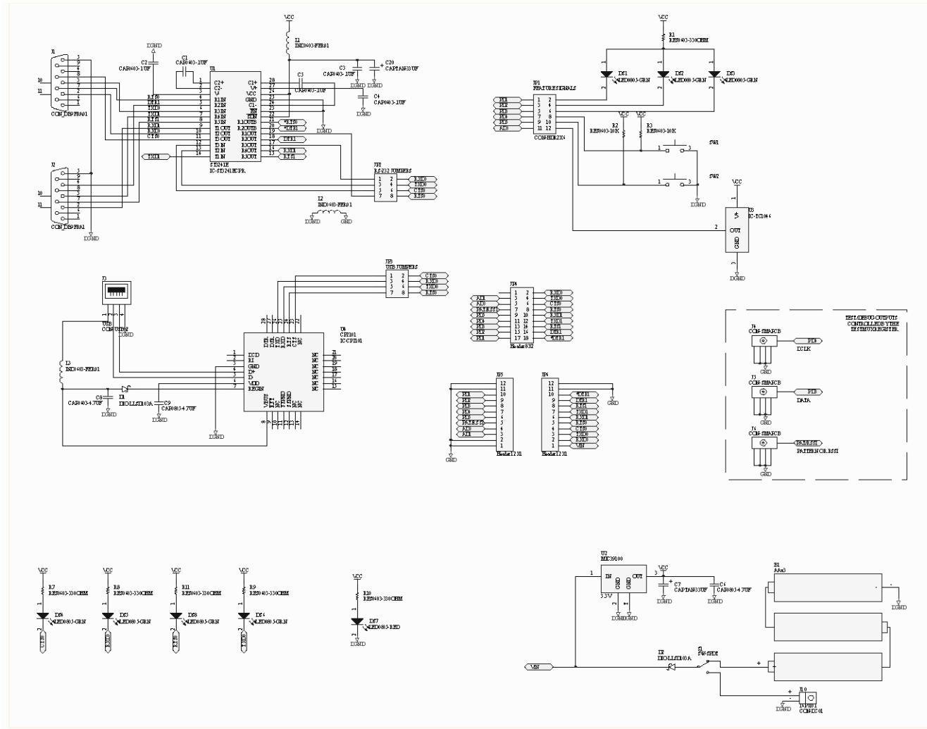
Figure 9: RK-WI.232EUR-R Evaluation Board Schematic Diagram
