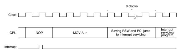
If an interrupt request flag (××IF) is set at the last clock of the instruction, the interrupt acknowledgment processing starts after the next instruction is executed.
