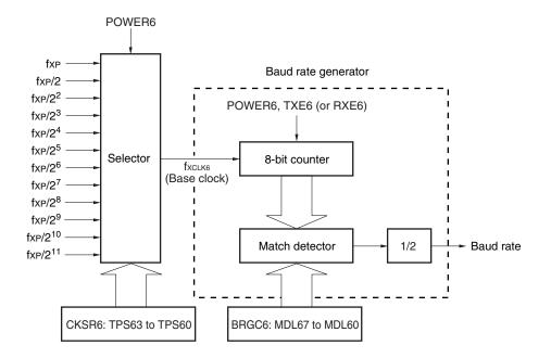
Figure 11-24. Configuration of Baud Rate Generator
