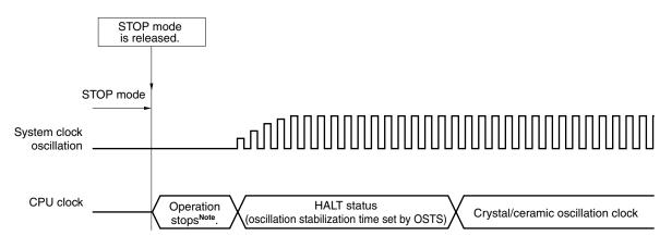
**Note** The operation stop time is 17  $\mu$ s (MIN.), 34  $\mu$ s (TYP.), and 67  $\mu$ s (MAX.).
