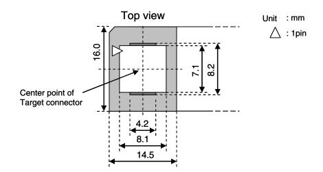
: Exchange adapter tip area  $\rightarrow$  Components up to 11.0 mm high can be mounted.
