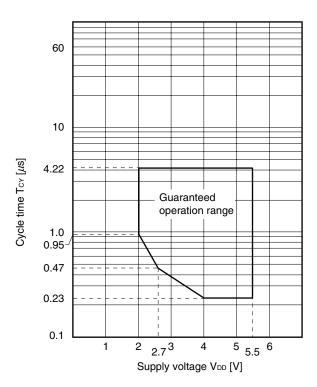
(2) Serial interface (T<sub>A</sub> = -40 to  $+85^{\circ}$ C, V<sub>DD</sub> = 2.0 to 5.5 V<sup>Note</sup>, V<sub>SS</sub> = 0 V)
