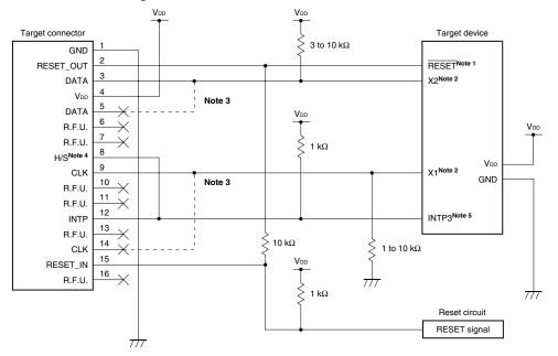
Figure 19-1. Recommended Circuit Connection
