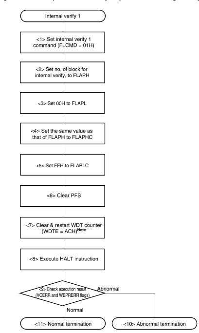
Figure 18-23. Example of Internal Verify 1 Operation in Self Programming Mode
