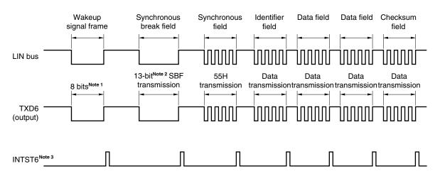
Figure 11-1. LIN Transmission Operation
