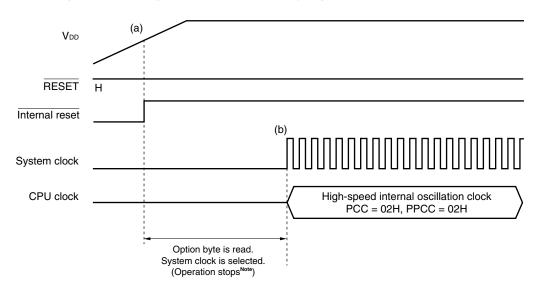
Figure 5-8. Timing Chart of Default Start by High-Speed Internal Oscillation
