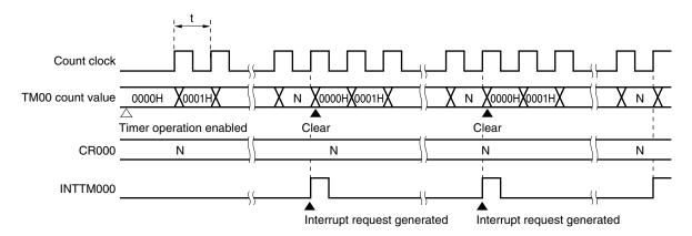
Figure 6-12. Timing of Interval Timer Operation
