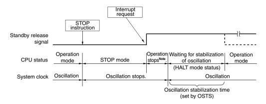
**Note** The operation stop time is 17  $\mu$ s (MIN.), 34  $\mu$ s (TYP.), and 67  $\mu$ s (MAX.).
