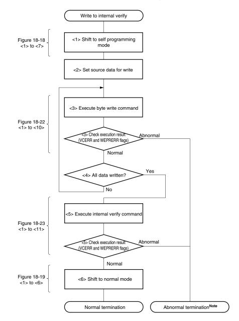
Note Perform processing to shift to normal mode in order to return to normal processing.
