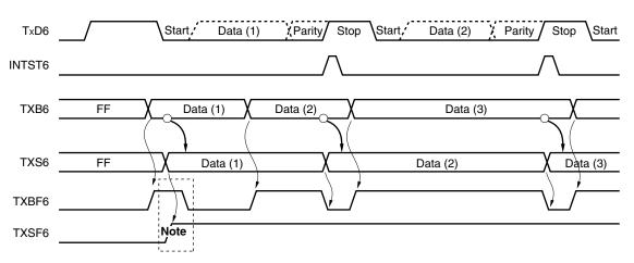
Figure 11-17. Timing of Starting Continuous Transmission
