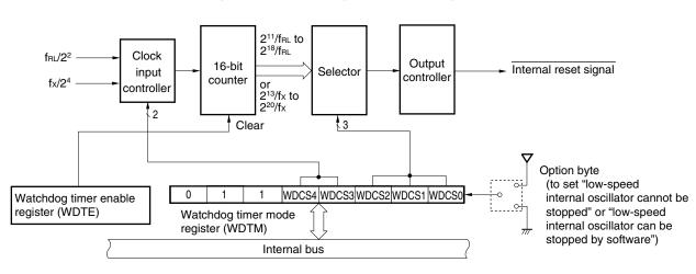
Figure 9-1. Block Diagram of Watchdog Timer
