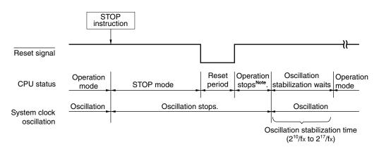
(2) If CPU clock is crystal/ceramic oscillation clock
