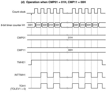
Figure 8-9. Operation Timing in PWM Output Mode (3/4)
