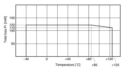
Use the following formula to perform design such that the sum of the power consumption of the device is less than or equal to the total loss  $P_T$  (use at 80% or less of the rated value is recommended).
