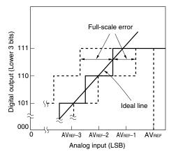
Figure 10-18. Differential Linearity Error
