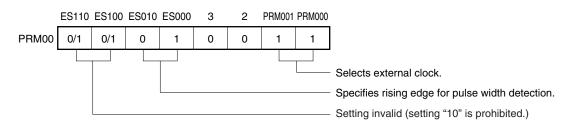
(c) 16-bit timer mode control register 00 (TMC00)
