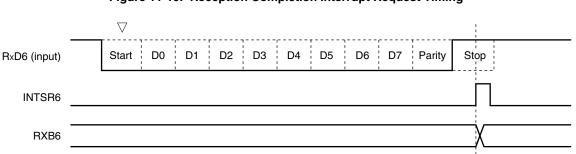
Figure 11-19. Reception Completion Interrupt Request Timing
