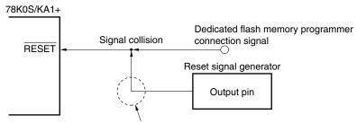
In the flash memory programming mode, the signal output by the reset signal generator collides with the signal output by the dedicated flash memory programmer. Therefore, isolate the signal of the reset signal
