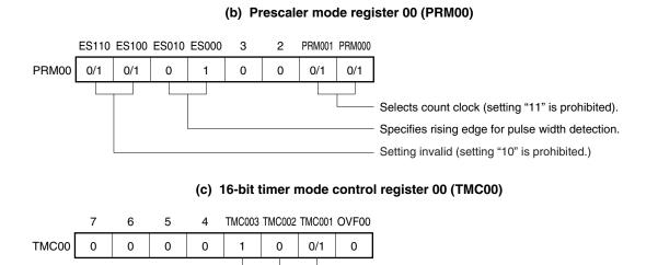
**Note** If the valid edge of TI000 pin is specified to be both the rising and falling edges, 16-bit timer capture/compare register 000 (CR000) cannot perform the capture operation.
