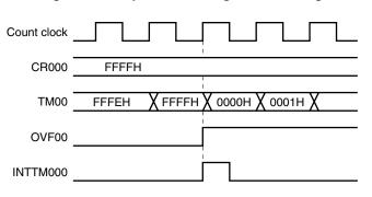
Figure 6-37. Operation Timing of OVF00 Flag
