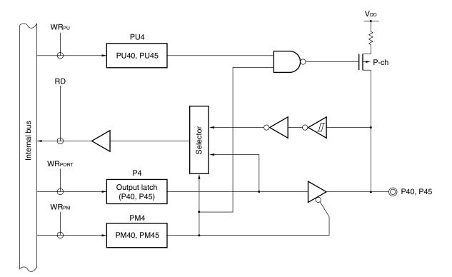
Figure 4-6. Block Diagram of P40 and P45
