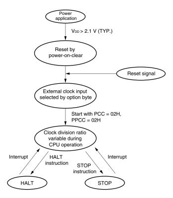
Remark PCC: Processor clock control register PPCC: Preprocessor clock control register
