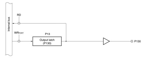
Figure 4-12. Block Diagram of P130
