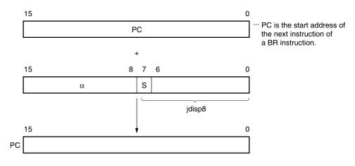
When S = 0,  $\alpha$  indicates that all bits are "0". When S = 1,  $\alpha$  indicates that all bits are "1".
