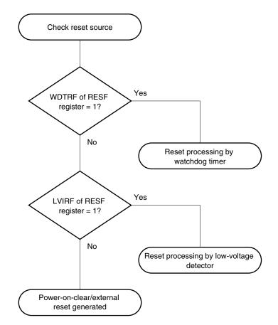
Figure 15-3. Example of Software Processing After Release of Reset (2/2)
