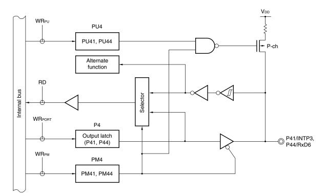
Figure 4-7. Block Diagram of P41 and P44
