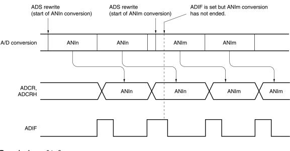
Figure 10-20. Timing of A/D Conversion End Interrupt Request Generation
