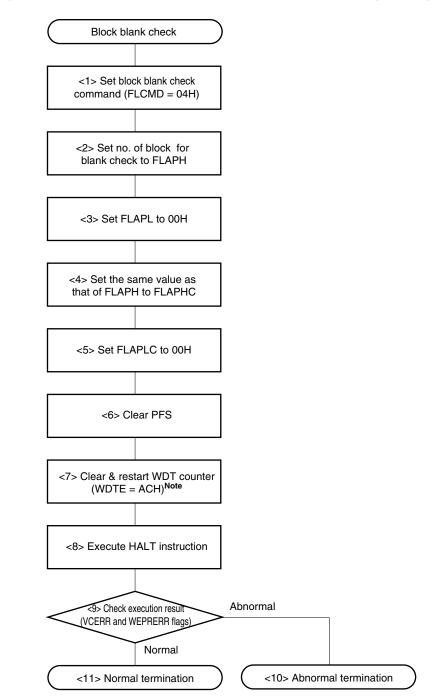
Figure 18-21. Example of Block Blank Check Operation in Self Programming Mode
