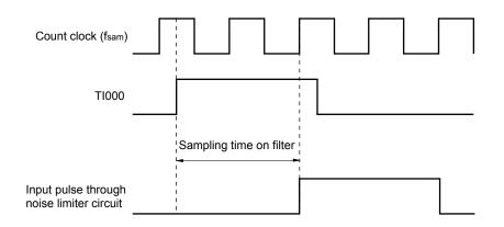
**Remark** The count clock (f<sub>sam</sub>) can be selected using bits 0 and 1 (PRM000, PRM001) of prescaler mode register 00 (PRM00).
