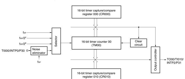
Figure 6-30. Configuration Diagram of PPG Output
