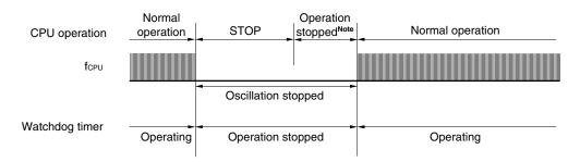
**Note** The operation stop time is 17  $\mu$ s (MIN.), 34  $\mu$ s (TYP.), and 67  $\mu$ s (MAX.).
