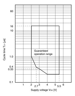
TCY vs. VDD (High-Speed Internal Oscillation Clock)
