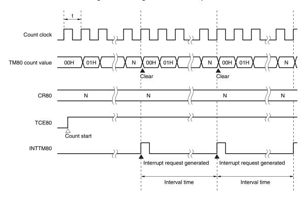
Figure 7-5. Timing of Interval Timer Operation
