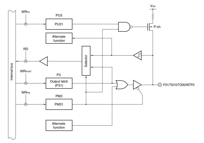
Figure 4-4. Block Diagram of P31
