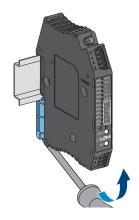
To remove the device, use a 4 mm flat screwdriver
