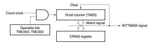
Figure 6-11. Block Diagram of Interval Timer Operation
