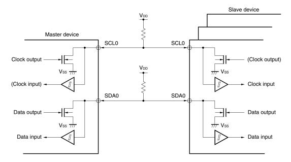
Figure 16-11. Pin Configuration Diagram
