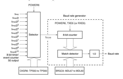
Figure 14-24. Configuration of Baud Rate Generator
