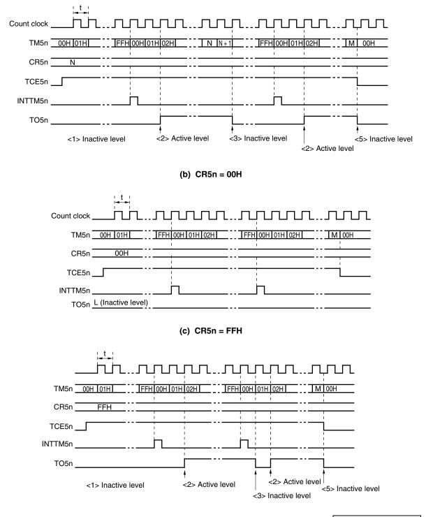
Remarks 1. <1> to <3> and <5> in Figure 7-14 (a) correspond to <1> to <3> and <5> in PWM output operation in 7.4.4 (1) PWM output basic operation.
