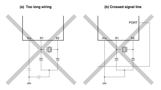
Figure 5-11. Examples of Incorrect Resonator Connection (1/2)
