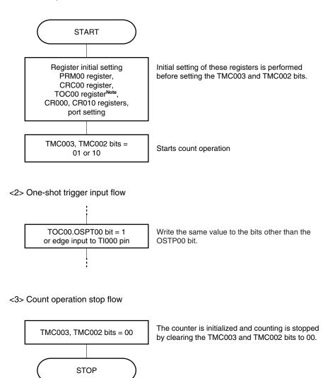
Note Care must be exercised when setting TOC00. For details, see 6.3 (3) 16-bit timer output control register 00 (TOC00).
