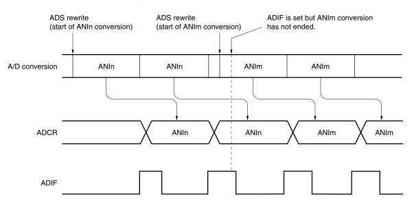
Figure 12-21. Timing of A/D Conversion End Interrupt Request Generation
