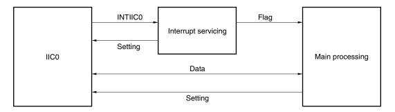
Therefore, data communication processing is performed by preparing the following three flags and passing them to the main processing instead of INTIIC0.
