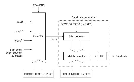
Figure 13-11. Configuration of Baud Rate Generator
