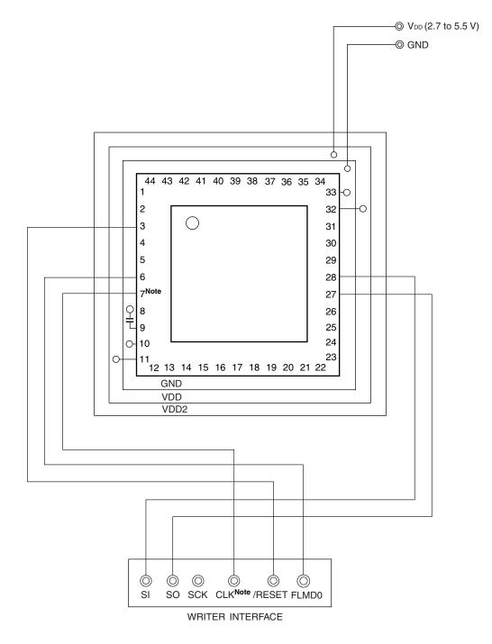
**Note** The above figure illustrates an example of wiring when using the clock output from the PG-FP4 or FL-PR4. When using the clock output from the PG-FPL3 or FP-LITE3, connect CLK to X1/P121 (pin 8), and connect its inverted signal to X2/EXCLK/P122 (pin 7).
