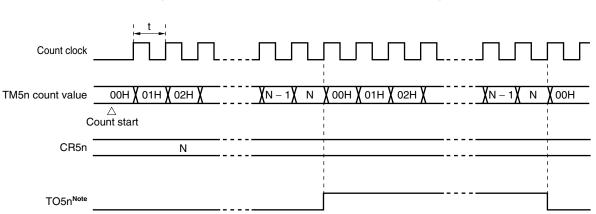
Figure 7-13. Square-Wave Output Operation Timing
