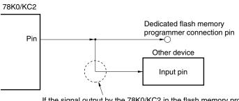
Figure 25-14. Malfunction of Other Device
