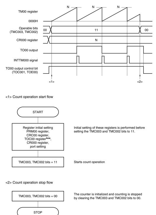
Note Care must be exercised when setting TOC00. For details, see 6.3 (3) 16-bit timer output control register 00 (TOC00).
