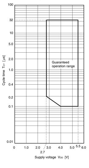
TCY vs. VDD (Main System Clock Operation)
