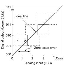
Figure 12-16. Zero-Scale Error
