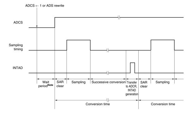
Figure 12-5. A/D Converter Sampling and A/D Conversion Timing
