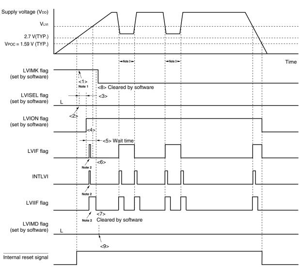
Figure 23-7. Timing of Low-Voltage Detector Interrupt Signal Generation (Detects Level of Supply Voltage (VDD)) (2/2)
