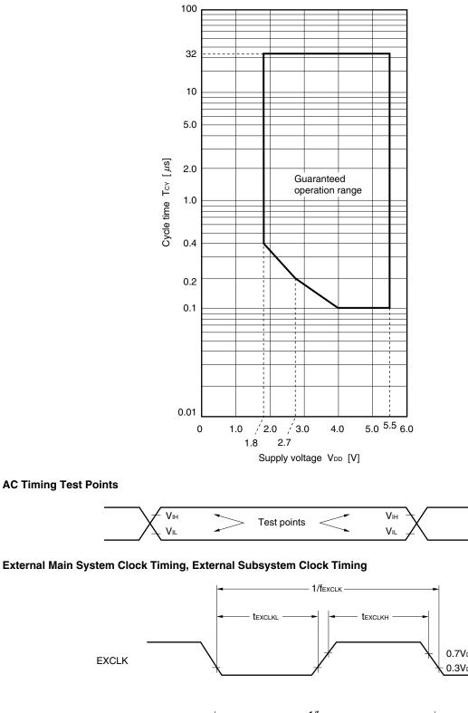
TCY vs. VDD (Main System Clock Operation)
