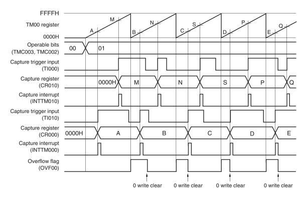
Figure 6-37. Timing Example of Free-Running Timer Mode (CR000: Capture Register, CR010: Capture Register) (1/2)
