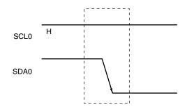
A start condition is output when bit 1 (STT0) of IIC control register 0 (IICC0) is set (to 1) after a stop condition has been detected (SPD0: Bit 0 = 1 in IIC status register 0 (IICS0)). When a start condition is detected, bit 1 (STD0) of IICS0 is set (to 1).
