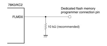
Figure 25-12. FLMD0 Pin Connection Example
