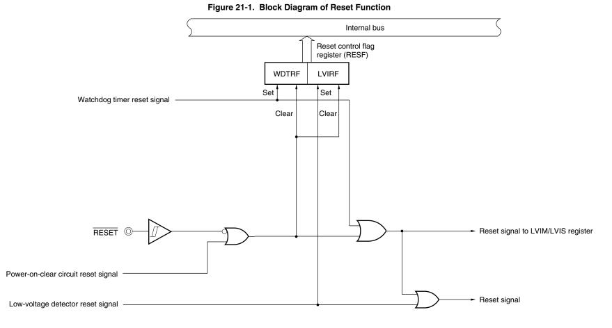
Caution An LVI circuit internal reset does not reset the LVI circuit.
