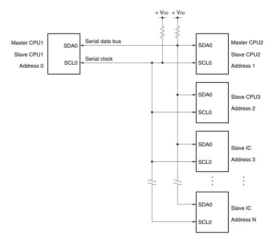
Figure 16-2. Serial Bus Configuration Example Using I<sup>2</sup>C Bus
