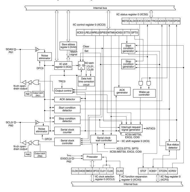
Figure 16-1. Block Diagram of Serial Interface IIC0
