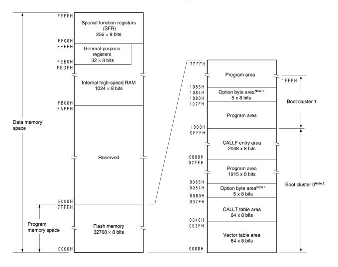
Notes 1. When boot swap is not used: Set the option bytes to 0080H to 0084H. When boot swap is used: Set the option bytes to 0080H to 0084H and 1080H to 1084H.
