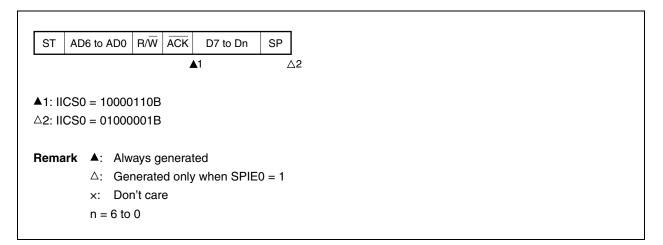
(f) When arbitration loss occurs due to low-level data when attempting to generate a restart condition
