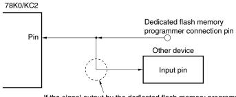
If the signal output by the dedicated flash memory programmer in the flash memory programming mode affects the other device, isolate the signal of the other device.
