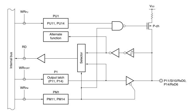
Figure 4-5. Block Diagram of P11 and P14
