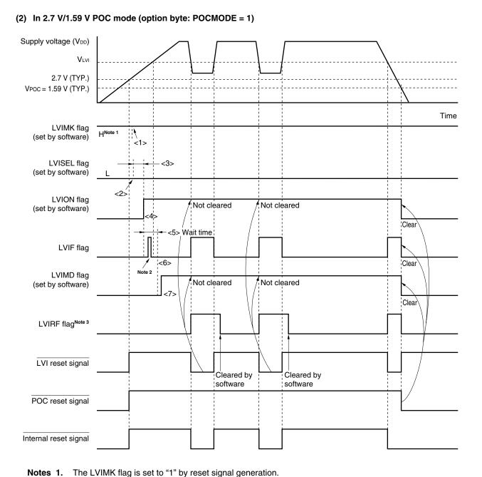
Figure 23-5. Timing of Low-Voltage Detector Internal Reset Signal Generation (Detects Level of Supply Voltage (VDD)) (2/2)
