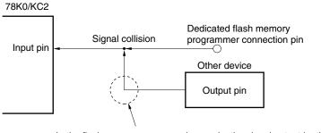
In the flash memory programming mode, the signal output by the device collides with the signal sent from the dedicated flash memory programmer. Therefore, isolate the signal of the other device.
