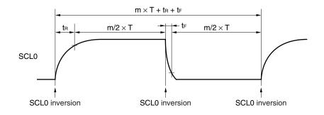
The selection clock is set using a combination of bits 3, 1, and 0 (SMC0, CL01, and CL00) of IIC clock selection register 0 (IICCL0) and bit 0 (CLX0) of IIC function expansion register 0 (IICX0).
