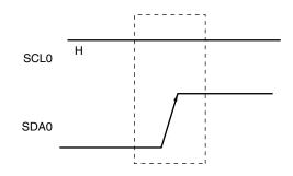
A stop condition is generated when bit 0 (SPT0) of IIC control register 0 (IICC0) is set to 1. When the stop condition is detected, bit 0 (SPD0) of IIC status register 0 (IICS0) is set to 1 and INTIIC0 is generated when bit 4 (SPIE0) of IICC0 is set to 1.
