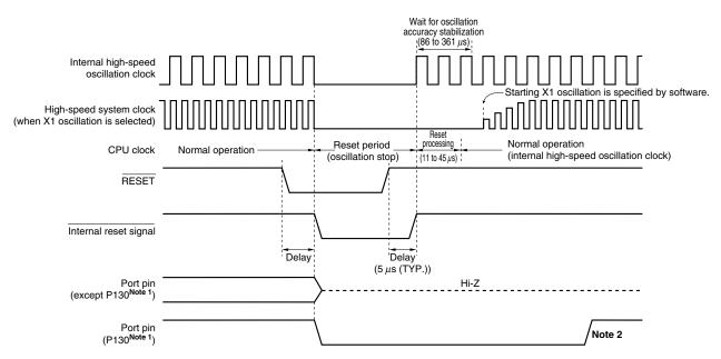
Figure 21-2. Timing of Reset by RESET Input
