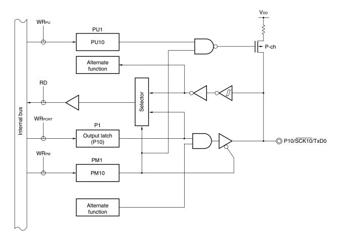
Figure 4-4. Block Diagram of P10
