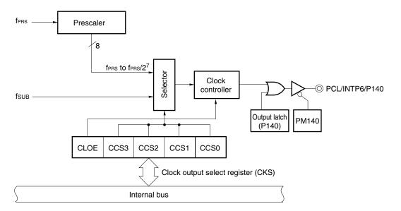
Figure 11-1. Block Diagram of Clock Output Controller
