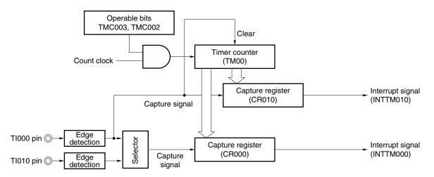
A pulse width can be measured in the following three ways.
