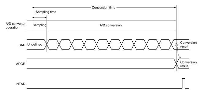
A/D conversion operations are performed continuously until bit 7 (ADCS) of the A/D converter mode register (ADM) is reset (0) by software.
