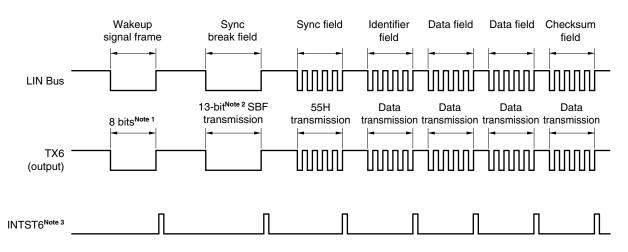
Figure 14-1. LIN Transmission Operation
