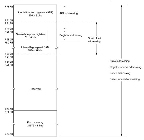
Figure 3-9. Correspondence Between Data Memory and Addressing (µPD78F0512)
