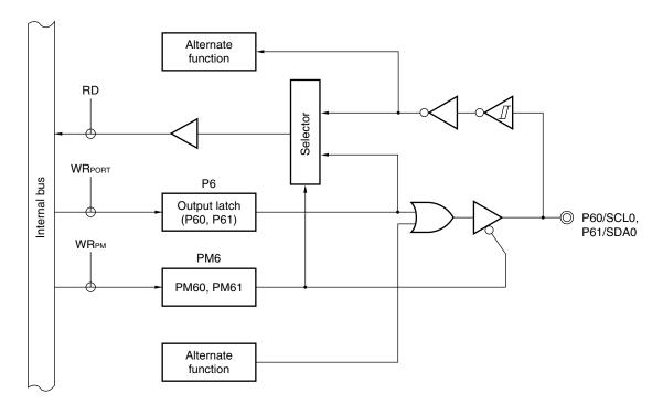
Figure 4-13. Block Diagram of P60 and P61
