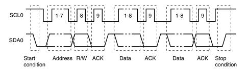
The master device generates the start condition, slave address, and stop condition.
