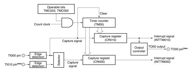
Note The timer output (TO00) cannot be used when detecting the valid edge of the TI010 pin is used.
