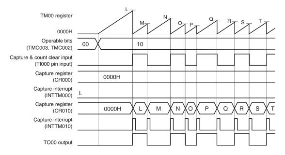
This is an application example where the count value is captured to CR010, TM00 is cleared, and TO00 output is inverted when the rising or falling edge of the TI000 pin is detected.
