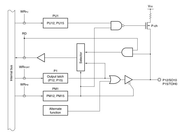
Figure 4-6. Block Diagram of P12 and P15
