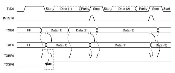
Figure 14-17. Timing of Starting Continuous Transmission
