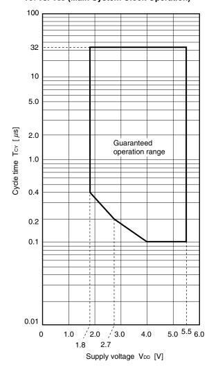
TCY vs. VDD (Main System Clock Operation)
