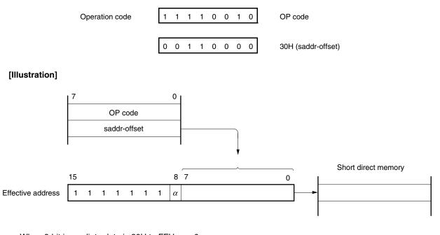
When 8-bit immediate data is 20H to FFH,  $\alpha = 0$ When 8-bit immediate data is 00H to 1FH,  $\alpha = 1$
