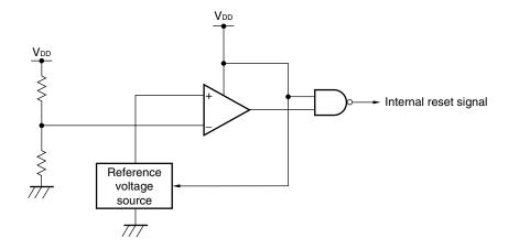
Figure 22-1. Block Diagram of Power-on-Clear Circuit
