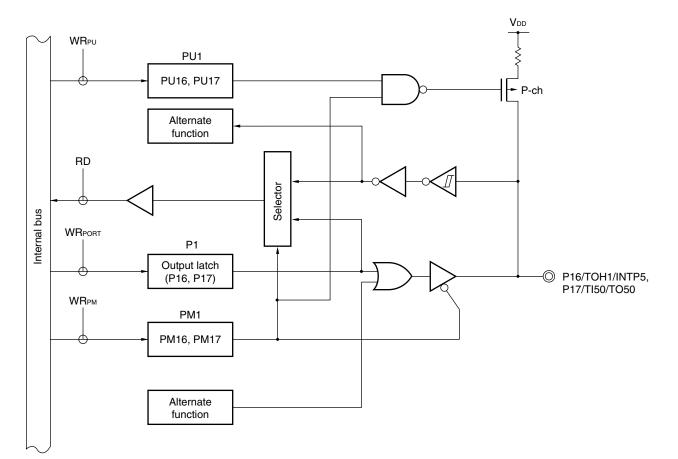
Figure 4-8. Block Diagram of P16 and P17
