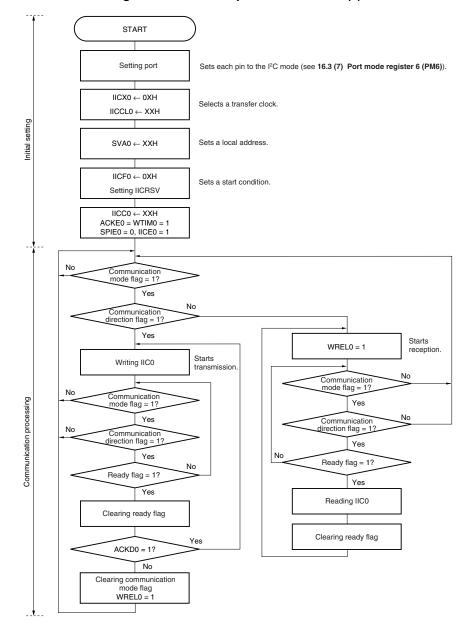
Figure 16-25. Slave Operation Flowchart (1)
