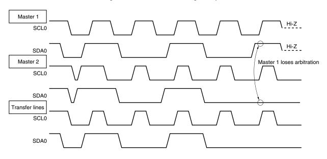
Figure 16-19. Arbitration Timing Example
