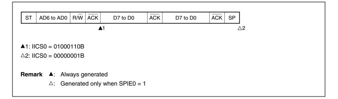
(b) When arbitration loss occurs during transmission of extension code
