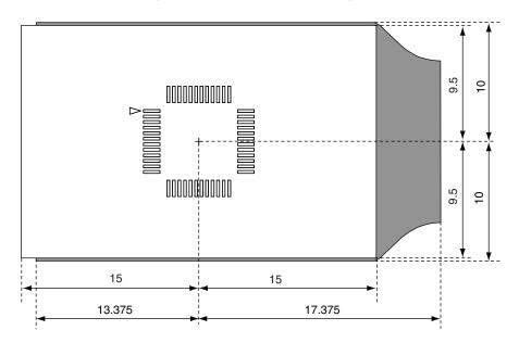
Exchange adapter area: Components up to 17.45 mm in height can be mounted<sup>Note</sup>
