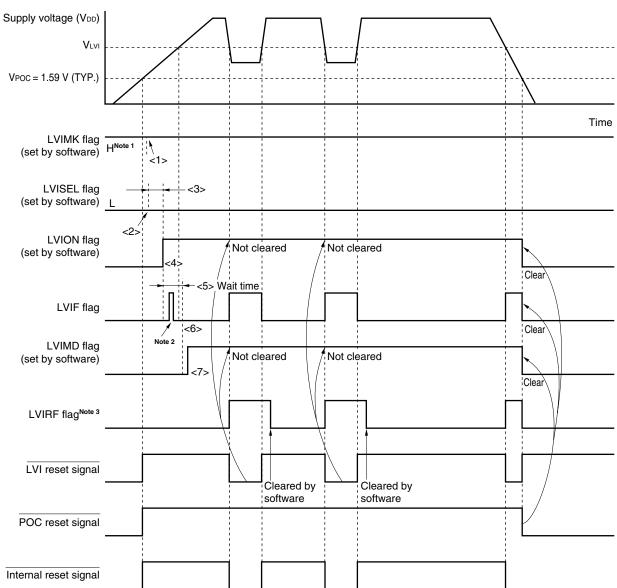
Figure 23-5. Timing of Low-Voltage Detector Internal Reset Signal Generation (Detects Level of Supply Voltage (VDD)) (1/2)
