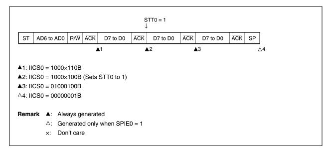
(g) When arbitration loss occurs due to a stop condition when attempting to generate a restart condition
