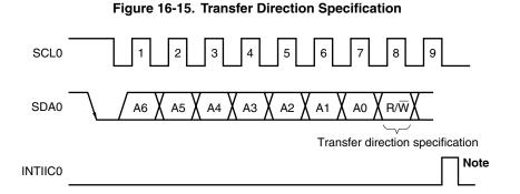
Note INTIIC0 is not issued if data other than a local address or extension code is received during slave device operation.
