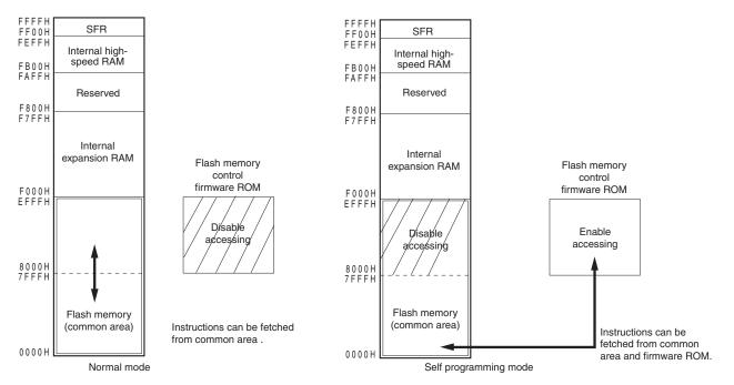
The following figure illustrates a flow of rewriting the flash memory by using a self programming library.
