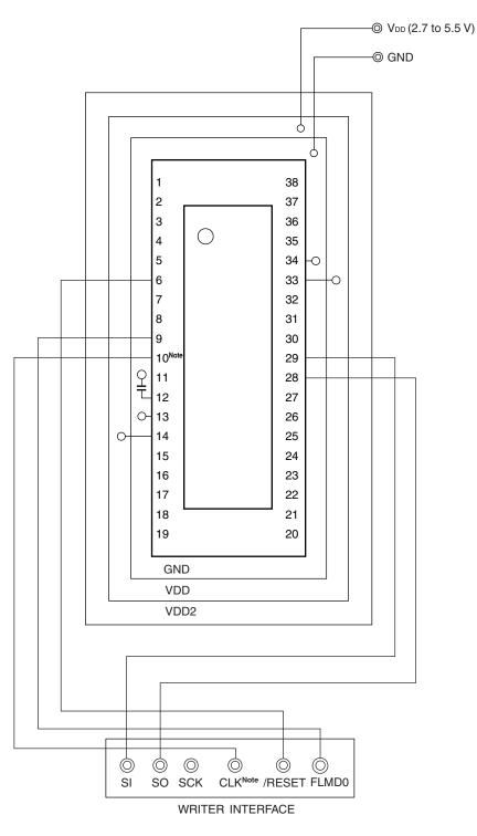
**Note** The above figure illustrates an example of wiring when using the clock output from the PG-FP4 or FL-PR4. When using the clock output from the PG-FPL3 or FP-LITE3, connect CLK to X1/P121 (pin 11), and connect its inverted signal to X2/EXCLK/P122 (pin 10).
