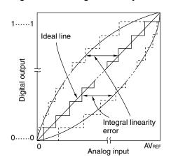
Figure 12-18. Integral Linearity Error
