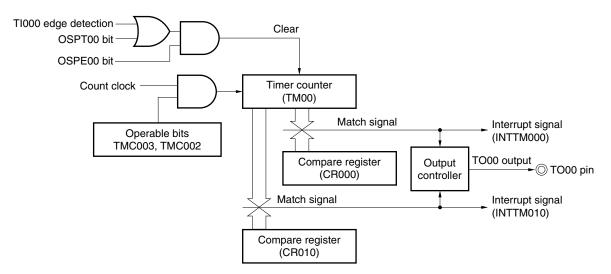
Figure 6-43. Block Diagram of One-Shot Pulse Output Operation
