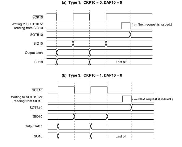
Figure 15-8. Output Value of SO10 Pin (Last Bit) (1/2)
