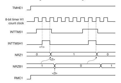
Figure 8-13. Transfer Timing
