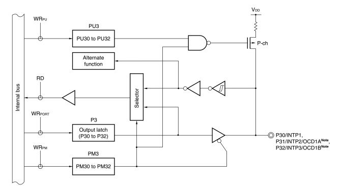
Figure 4-10. Block Diagram of P30 to P32
