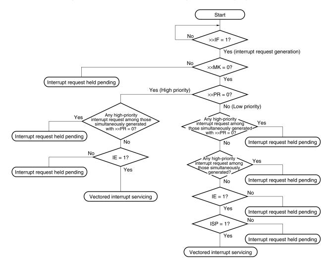
Figure 18-7. Interrupt Request Acknowledgment Processing Algorithm
