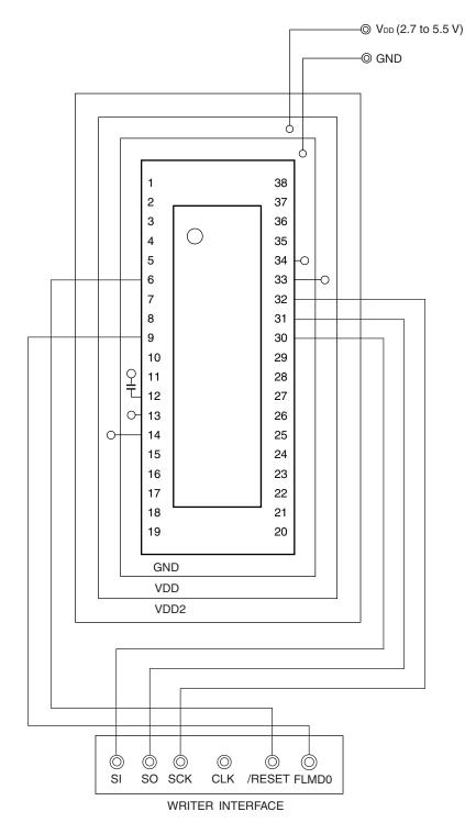
Figure 25-4. Example of Wiring Adapter for Flash Memory Writing in UART (UART6) Mode (38-Pin Products)
