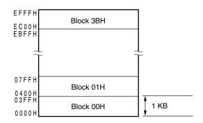
Correspondence between the address values and block numbers in the flash memory are shown below.
