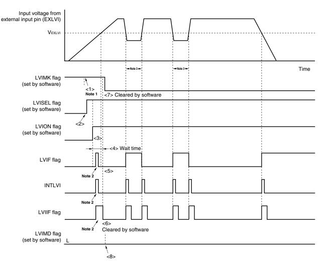
Figure 23-8. Timing of Low-Voltage Detector Interrupt Signal Generation (Detects Level of Input Voltage from External Input Pin (EXLVI))
