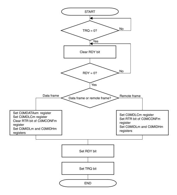
Figure 16-42. Message Transmit Processing
