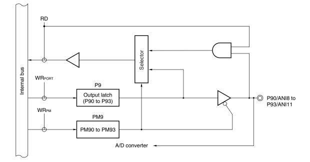
Figure 5-18. Block Diagram of P90 to P93
