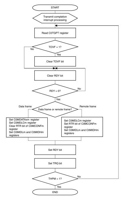
Figure 16-45. Transmit via Interrupt (Using C0TGPT register)
