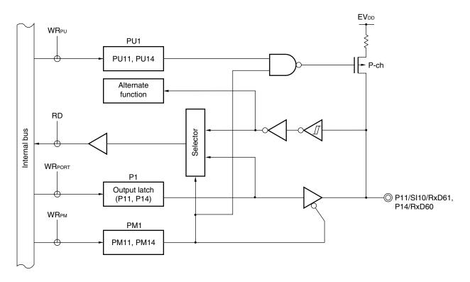
Figure 5-5. Block Diagram of P11 and P14
