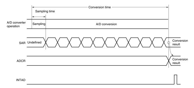
Figure 13-12. Basic Operation of A/D Converter
