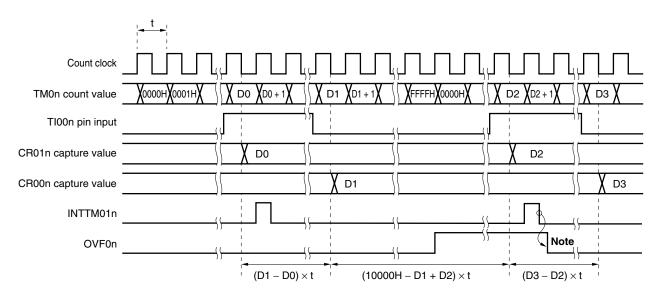
Figure 7-41. Timing of Pulse Width Measurement Operation with Free-Running Counter and Two Capture Registers (with Rising Edge Specified)
