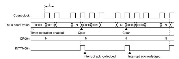
Figure 7-30. Timing of Interval Timer Operation
