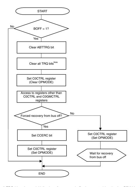
Figure 16-57. Bus-Off Recovery (Normal Operation Mode with ABT)
