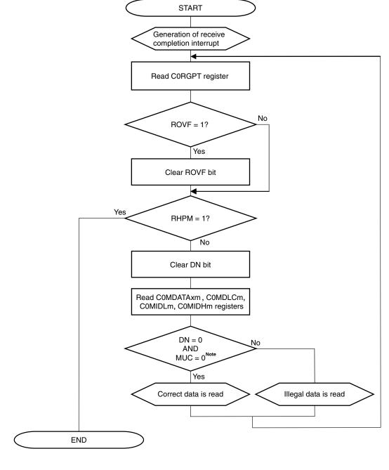
Figure 16-52. Reception via Interrupt (Using C0RGPT Register)
