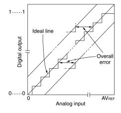
Figure 13-16. Quantization Error
