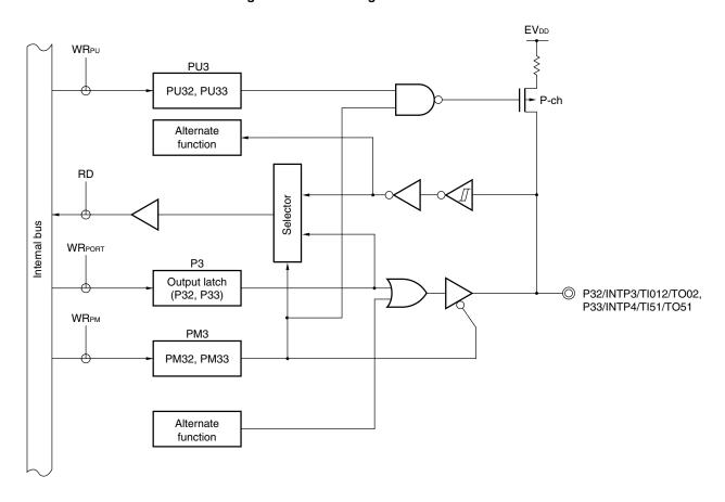
Figure 5-8. Block Diagram of P32 and P33
