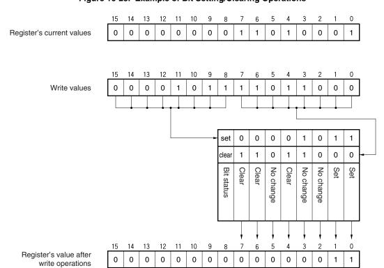
Figure 16-24. 16-Bit Data during Write Operation
