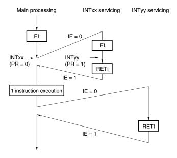
Figure 17-10. Examples of Multiple Interrupt Servicing (2/2)
