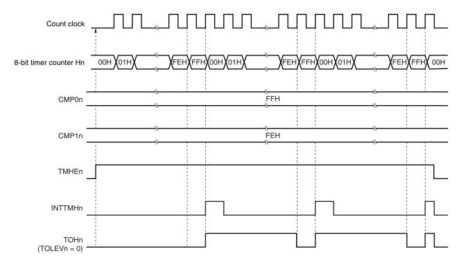
Figure 9-12. Operation Timing in PWM Output Mode (3/4)
