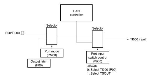
Figure 16-36. Port Input Switch Control
