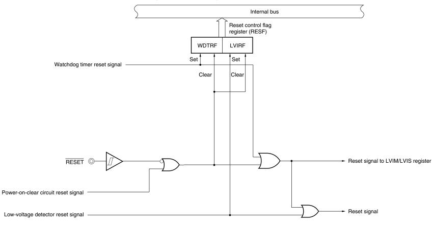
Figure 19-1. Block Diagram of Reset Function
