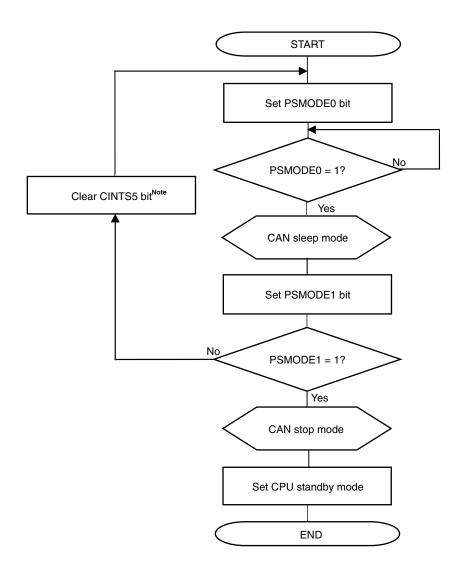
Figure 16-62. Setting CPU Standby (from CAN Stop Mode)
