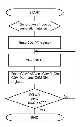
Figure 16-51. Reception via Interrupt (Using C0LIPT Register)
