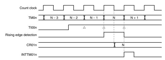
Figure 7-34. CR01n Capture Operation with Rising Edge Specified
