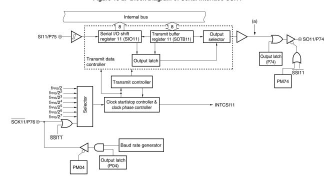
Figure 15-2. Block Diagram of Serial Interface CSI11
