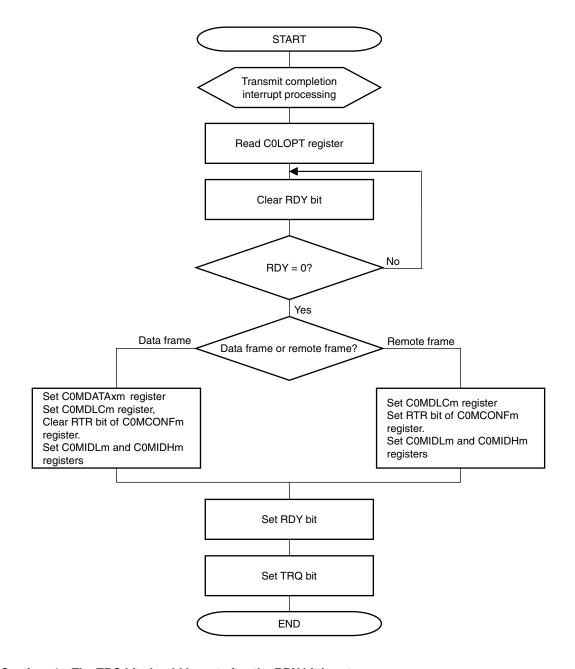
Figure 16-44. Transmission via Interrupt (Using C0LOPT register)
