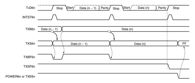
Figure 14-26. Timing of Ending Continuous Transmission
