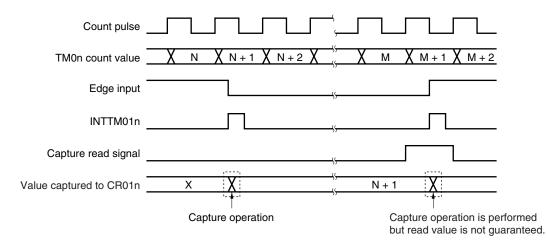
Figure 7-56. Timing of Holding Data by Capture Register
