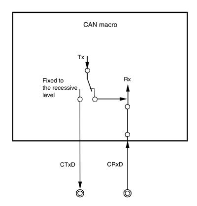
Figure 16-33. CAN Module Terminal Connection in Receive-Only Mode
