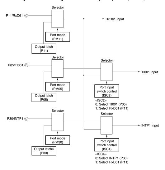
Figure 14-4. Port Configuration for LIN Reception Operation (UART61)
