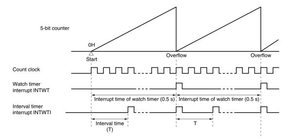
Figure 10-3. Operation Timing of Watch Timer/Interval Timer
