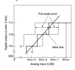
Figure 13-20. Differential Linearity Error
