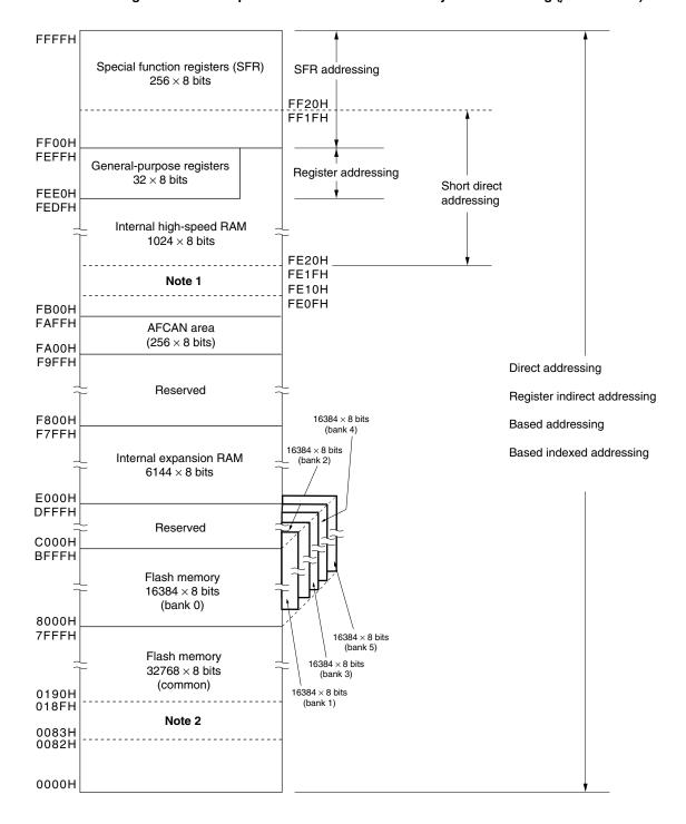
Figure 3-9. Correspondence Between Data Memory and Addressing (μPD78F0890)
