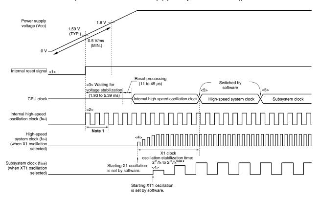
Figure 6-12 Operation of the clock generating circuit when power supply voltage injection (When 1.59 V POC mode setup (option byte: LVISTART = 0))
