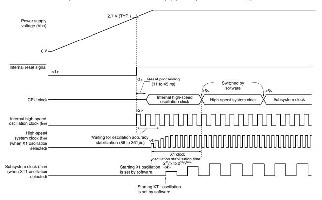
Figure 6-13 Operation of the clock generating circuit when power supply voltage injection (When 2.7 V/1.59V POC mode setup (option byte: LVISTART = 1))
