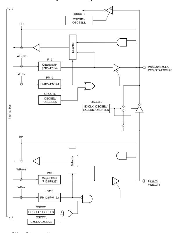
Figure 5-20. Block Diagram of P121 to P124
