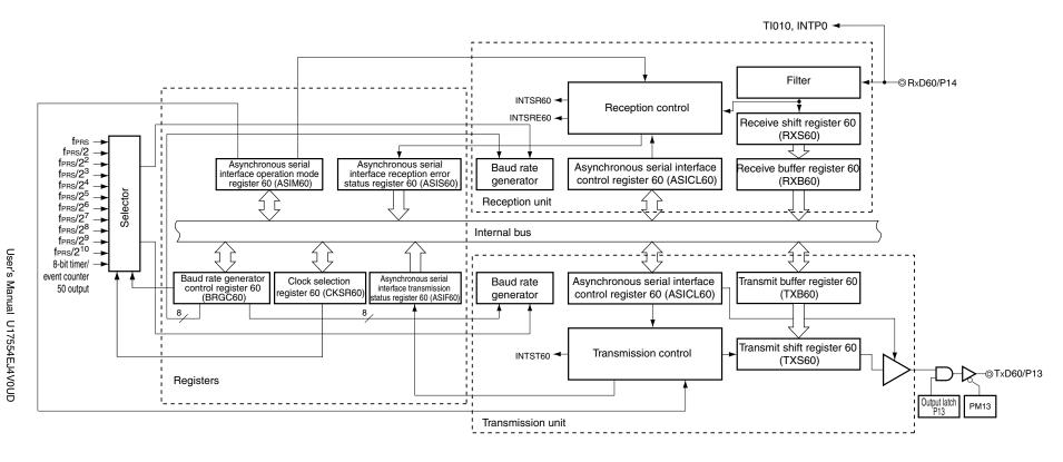
Figure 14-5. Block Diagram of Serial Interface UART60
