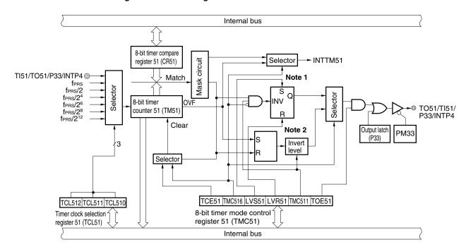
Figure 8-2. Block Diagram of 8-Bit Timer/Event Counter 51
