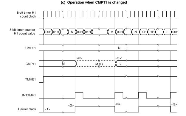
Figure 9-15. Carrier Generator Mode Operation Timing (3/3)
