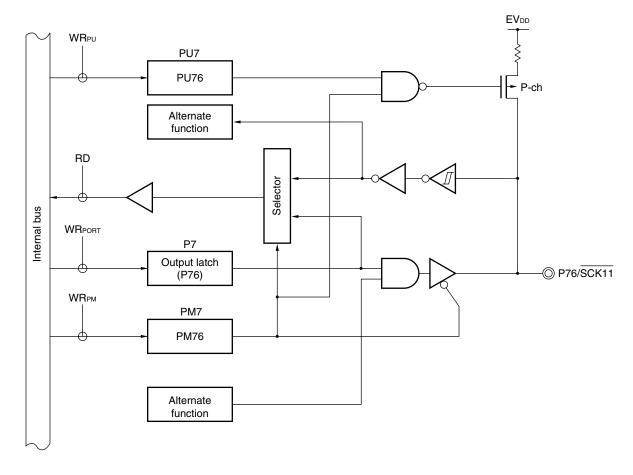
PU7: Pull-up resistor option register 7
