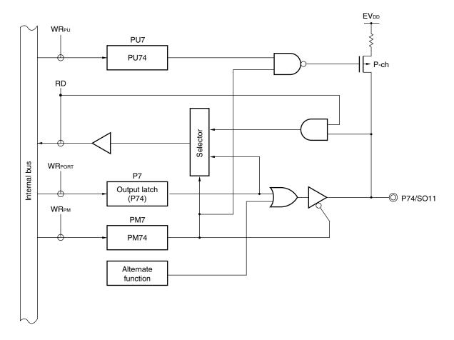
PU7: Pull-up resistor option register 7
