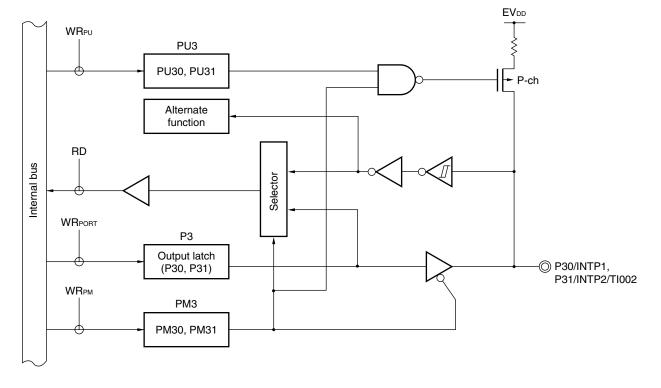
Figure 5-7. Block Diagram of P30 and P31
