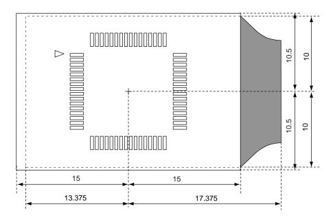
: Exchange adapter area: Components up to 17.45 mm in height can be mounted Note
