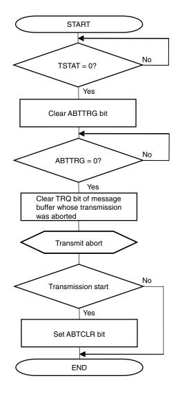
Figure 16-49. ABT Transmission Abort Processing (Normal Operation Mode with ABT)
