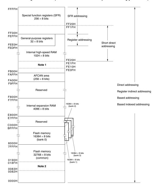
Figure 3-8. Correspondence Between Data Memory and Addressing (μPD78F0889)
