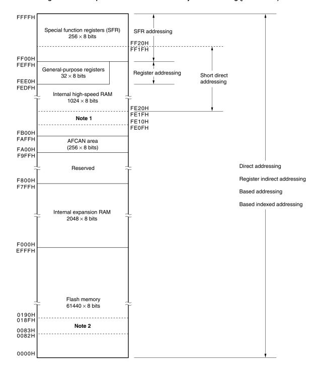
Figure 3-7. Correspondence Between Data Memory and Addressing (μPD78F0888)
