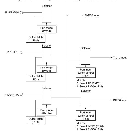
Figure 14-3. Port Configuration for LIN Reception Operation (UART60)
