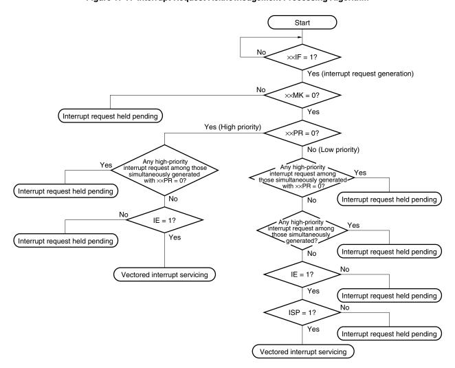
Figure 17-7. Interrupt Request Acknowledgement Processing Algorithm
