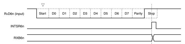
Figure 14-27. Reception Completion Interrupt Request Timing
