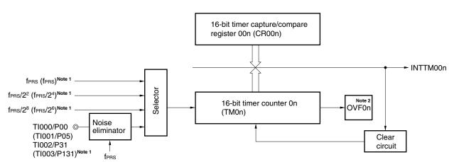
Figure 7-29. Interval Timer Configuration Diagram
