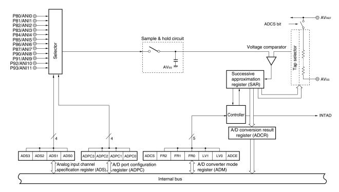
Figure 13-1. Block Diagram of A/D Converter
