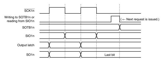
Figure 15-13. Output Value of SO1n Pin (Last Bit) (2/2)
