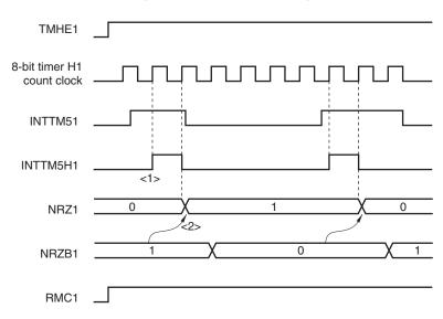
Figure 9-13. Transfer Timing
