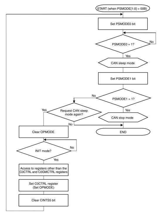
Figure 16-54. Setting CAN Sleep Mode/Stop Mode
