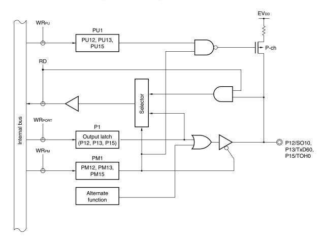
Figure 5-6. Block Diagram of P12, P13 and P15
