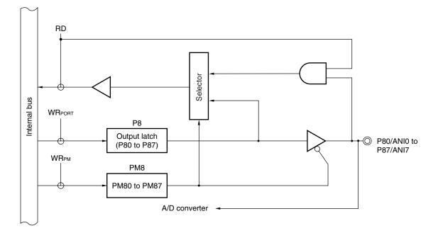
Figure 5-17. Block Diagram of P80 to P87
