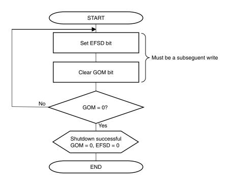
Figure 16-59. Forced Shutdown Process
