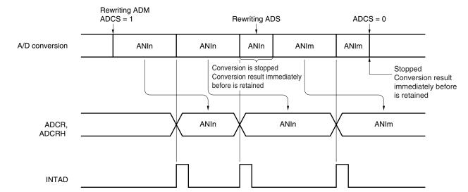
Figure 13-14. A/D Conversion Operation
