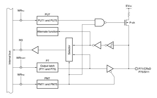
Figure 5-13. Block Diagram of P71 and P75
