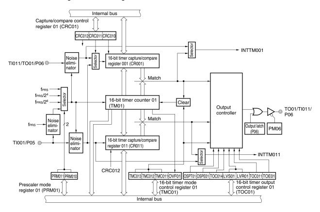
Figure 7-2. Block Diagram of 16-Bit Timer/Event Counter 01
