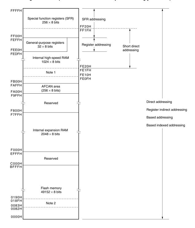
Figure 3-6. Correspondence Between Data Memory and Addressing (µPD78F0887)
