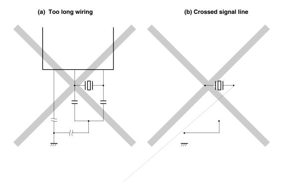
Figure 6-11. Examples of Incorrect Resonator Connection (2/2)
