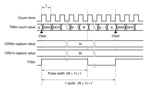
Figure 7-33. PPG Output Operation Timing
