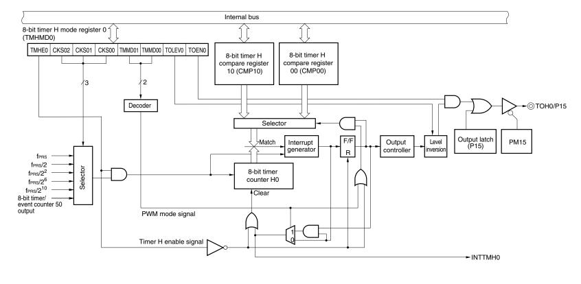
Figure 9-1. Block Diagram of 8-Bit Timer H0
