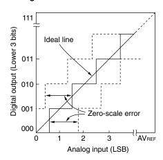
Figure 13-19. Integral Linearity Error
