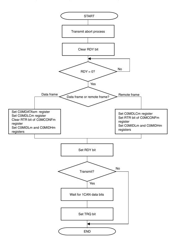
Figure 16-41. Message Buffer Redefinition during Transmission
