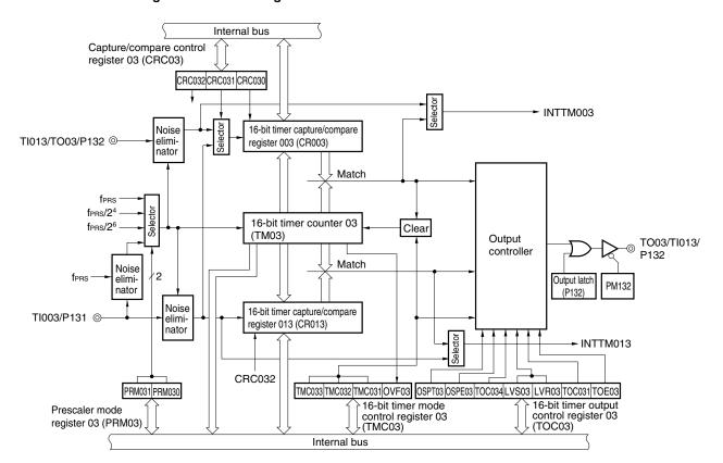
Figure 7-4. Block Diagram of 16-Bit Timer/Event Counter 03
