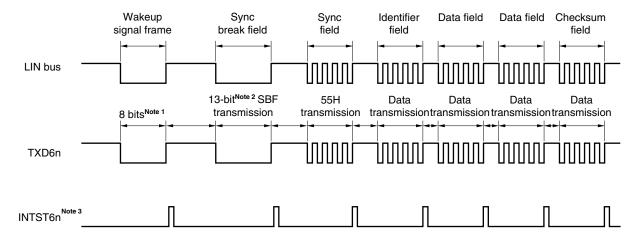
Figure 14-1. LIN Transmission Operation
