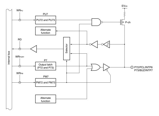
PU7: Pull-up resistor option register 7
