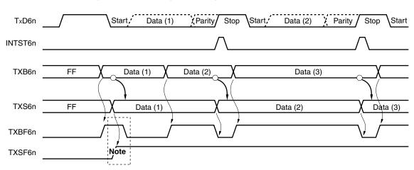
Figure 14-25. Timing of Starting Continuous Transmission
