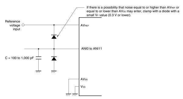
Figure 13-21. Analog Input Pin Connection
