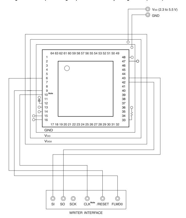
Figure 24-4. Example of Wiring Adapter for Flash Memory Writing in UART (UART60) Mode
