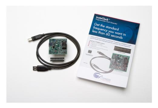
The CY36800 InstaClock Universal Programmable Clock Generator Development Kit contains the programming board with a USB cable, and 3 samples each of the CY22800 and CY22801 devices. The latest programming software is available to download from www.cypress.com/instaclock.
