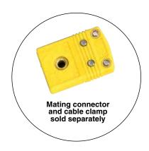
Omega™ miniature dual element thermocouple probe assemblies are manufactured using 4-conductor OMEGACLAD™ wire, and feature SMP subminiature connectors for fast hook-up. 304 stainless steel sheaths are standard, with either 1.5 mm (0.062") or 3 mm 0.125" OD Junctions are either grounded, ungrounded or exposed. Mating connector and cable clamp sold separately. Standard length is 150 mm (6"), with other lengths available.
