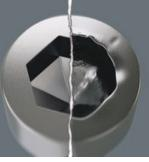
Hexagon screws can endure a because the contact problem surfaces delivering the power from the conventional tool, is transferred to the screw via very small surface areas. The consequence: the screw can become damaged (rounding out). Hex-Plus tools have a greater contact surface that prevents this from happening! At the same time, as much as 20 % more torque can be applied. Good to know: Hex-Plus tools fit into every standard hexagon socket screw!
